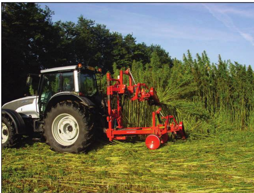
FIGURE 7.37 Specialized equipment required for harvesting tall C. sativa grown for stem fiber in France. Photo by Aleks (CC BY 3.0).
