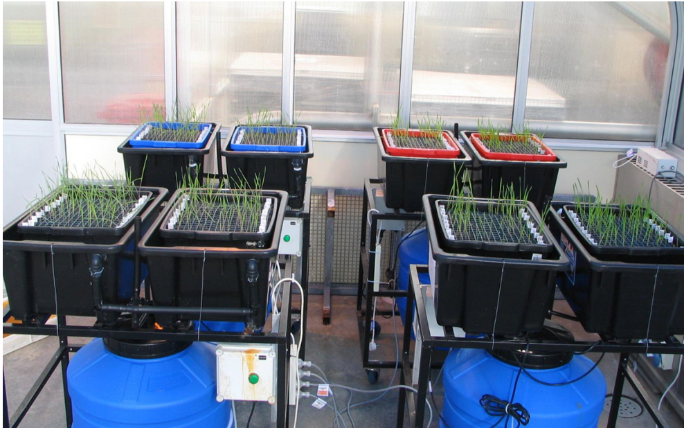
Fig. 1. A flood-drain 80 L supported hydroponics system in use at the Australian Centre for Plant Functional Genomics (ACPFPG).
