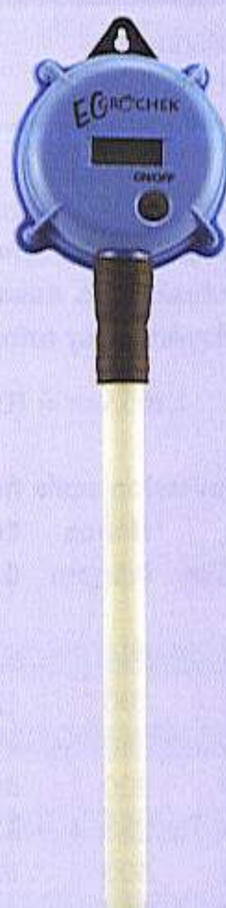
ABOVE RIGHT: Constant read-out, temperature-compensated EC/ppm meters with a probe immersed in the nutrient tank provide round-the-clock intelligence.
