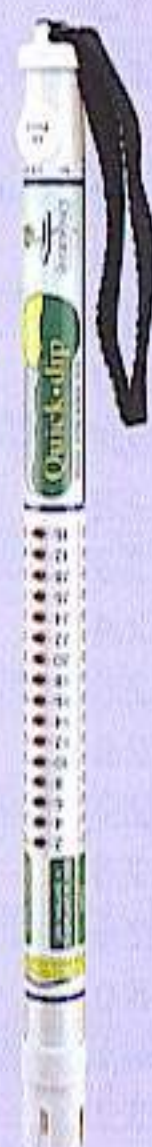
ABOVE RIGHT: Constant read-out, temperature-compensated EC/ppm meters with a probe immersed in the nutrient tank provide round-the-clock intelligence.
