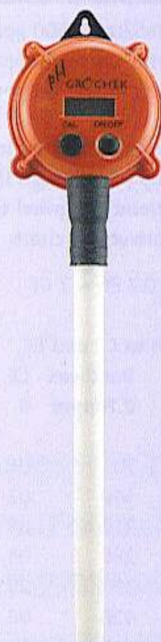
ABOVE LEFT: The probe of this meter is submerged in the nutrient solution to monitor pH 24 hours a day.
