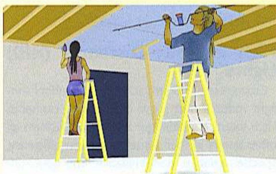
Affix a sturdy board to the ceiling. Mount a light mover on the board with joist below. Run electrical cord via timer to light mover.
