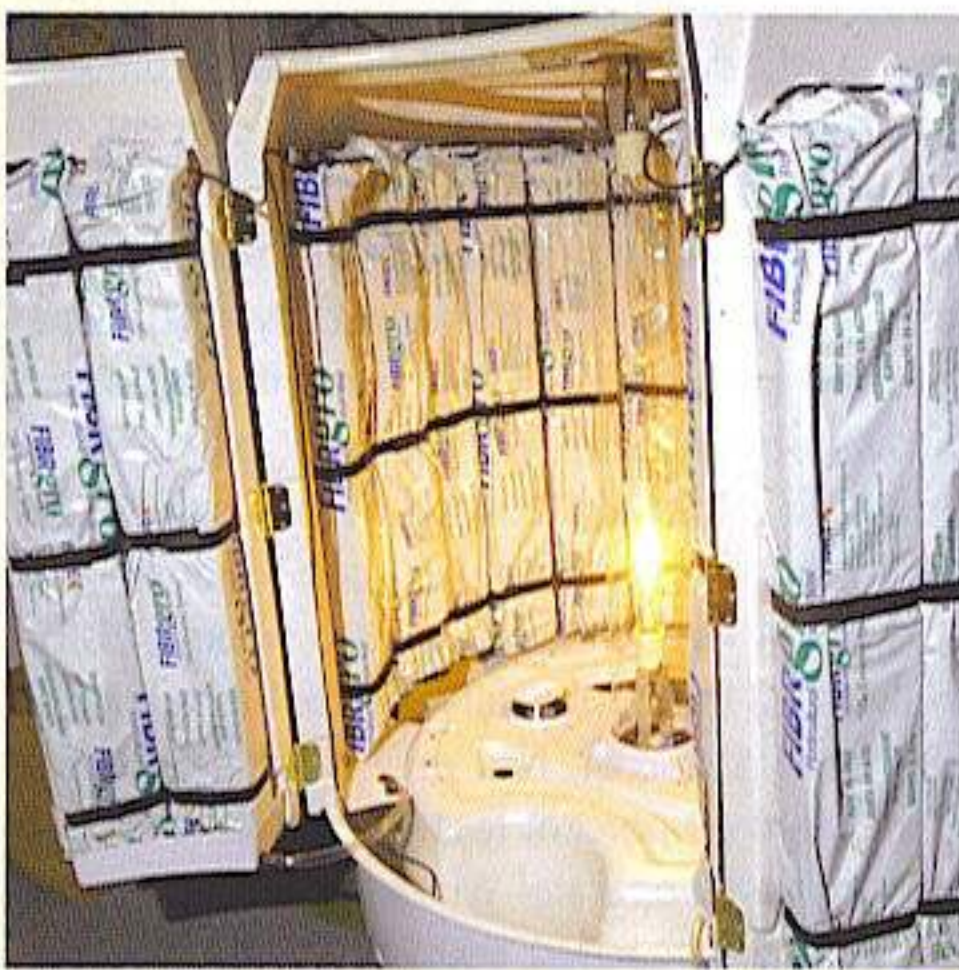
Plants grow in vertical slabs and are irrigated from above in this recirculating garden.
